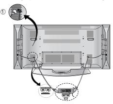
Place the speakers in the position you want. Install the speaker wires on the TV and speaker. Be sure to connect the positive "+" wire to the "+" input and the negative "-" wire to the "-" input. Connect left monitor input to left speaker and right monitor input to right speaker. Any extra speaker wire length remaining can be bunched into the wire holders provided, see (1) above to install wire holders. (Caution: Once installed, the speaker wire holders lock into position and can't be removed.)
